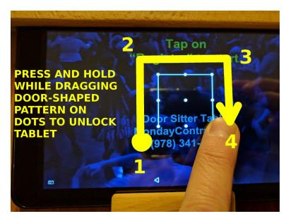
Touch and hold on the screen as you trace the path of the door pattern on the screen as shown. Once correctly entered, the tablet will be unlocked and ready for use.
