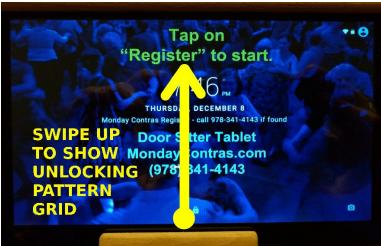
Once the screen is on, swipe up with your finger from the bottom of the screen near the lock icon to get the 9 dot security pattern to show. (You may not need to do this, skip ahead to the matching screen you encounter.)
