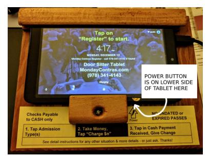
The power switch is the smaller of the two buttons on the bottom long side of the tablet (switch position is indicated on the tablet stand). Press it once to turn on the screen.
